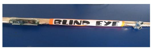
The smart stick for the blind as the name suggests is a device for the visually impaired to guide the user to respective destination and avoiding to collide with the obstacles. It uses two ultrasonic sensors HC SR 04 to detect the depth below or the obstacles in between.
